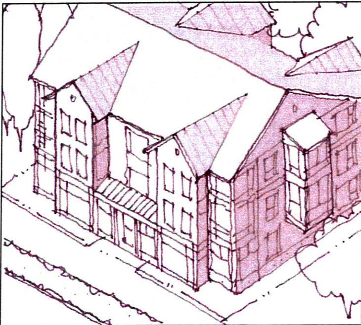
Bays, dormers, balconies and other projected or recessed design elements reduce the building's mass and add visual interest
